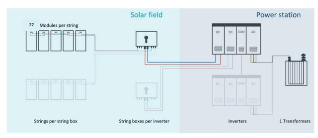
Figure 7. Simplified electrical configuration diagram
