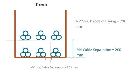
Figure 15. Simplified MV trench cross section
