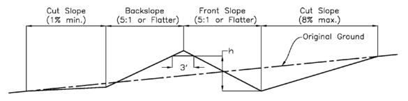
Length of front slope and backslope shall be in increments of machinery width but not less than 15 feet h = Design height of the terrace
