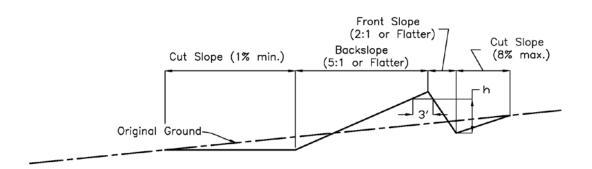
Length of backslope shall be in increments of machinery width but not less than 15 feet h = Design height of the terrace
