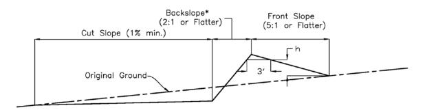
Length of front slope shall be in increments of machinery width but not less than 15 feet \*The backslope shall be no steeper than 2:1 except when built on Ida and Monona soil series types which may have the backslope constructed no steeper than 1.5:1 h = Design height of the terrace
