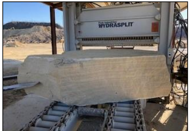
The center stone or “cairn”, was cut and then hand shaped from natural bed limestone at the quarry in Stone City and then transported and set in place. The stone marks the exact center of lines marking the sunrise and sunset on the horizon during the solstices and equinox’s. The stone weighs approximately 9,500 lbs.
