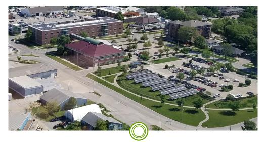
In 2016, the County nearly quadrupled solar-generated electricity for its facilities by adding an 86 kW ground-mounted array to the Administration Building and a 159 kW roof-top array to the Health and Human Services Building.
